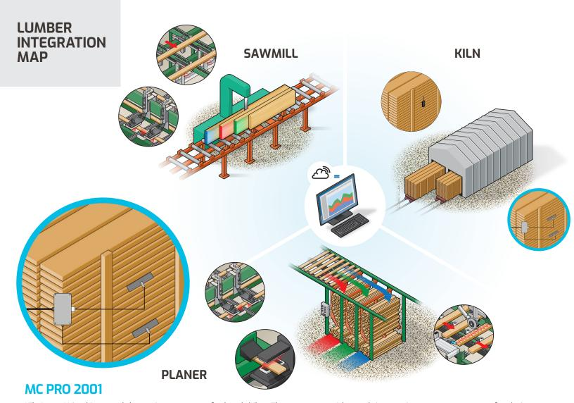
KilnScout-Wired is a modular moisture system for batch kilns. The system provides real-time moisture measurements for drying optimization and control strategies. Each sensor measures 17 cubic feet providing an accurate representation of product moisture content during drying. Data is integrated with planer systems for advanced reporting and drying analysis.
